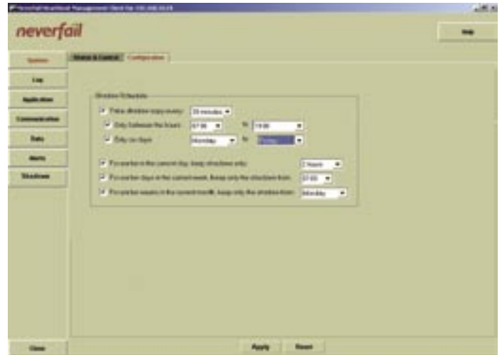
The Configuration Panel allows IT administrators to set the time granularity/intervals of shadow copies.
