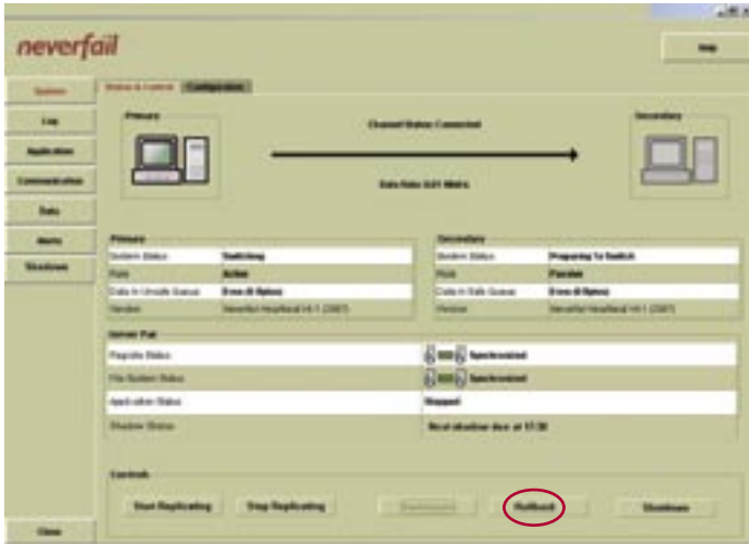
Neverfail interface incorporates the Data Rollback feature; allowing for data to be rolled back to a previous point in time at the click of a button.
